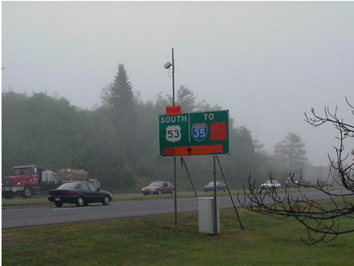
Fig. 2 The side-fired mounted RTMS detector at location # 4 close to Cottonwood Avenue.
