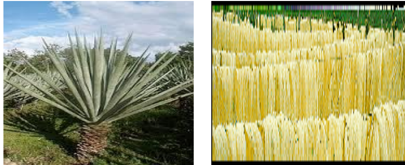
Figure2: Showing example of sisal leaf plant and the fiber after decortications (Adapted from: Tara and Jagannatha, 2011)
